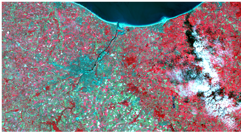
Fig. 9 Landsat-8 image taken on the 17 th of July 2013 – red displays near-infrared, green displays red and blue displays green (traditional false-color composite). Contains USGS/NASA Landsat Program data © 2013 processed at level 2A by CNES for THEIA Land data centre.
